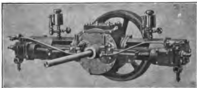
FIG. 394. —Double Opposed Horizontal Cylinder Motor of the Haynes-Apperson Carriages. The two cylinders of this motor are somewhat offset, as shown in the cut, the crank rods working on two cranks. The long crank shaft shown at the front of the engine is for carrying the change speed gear already described. The reciprocating parts are lubricated by adjustable oil feed cups shown at the top of each cylinder. Ignition is by break contact spark, the exhaust connections being on the same plan as those described for other motors.
